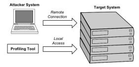
Figure 1. Experimental setup for profiling data collection
