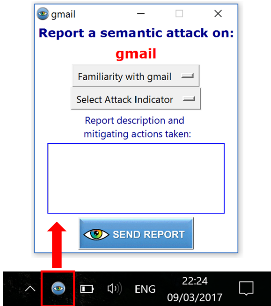
Figure 6: The Cogni-Sense HaaSS reporting app icon running in system tray. When clicked, a reporting window is opened with the detected platform and report information
