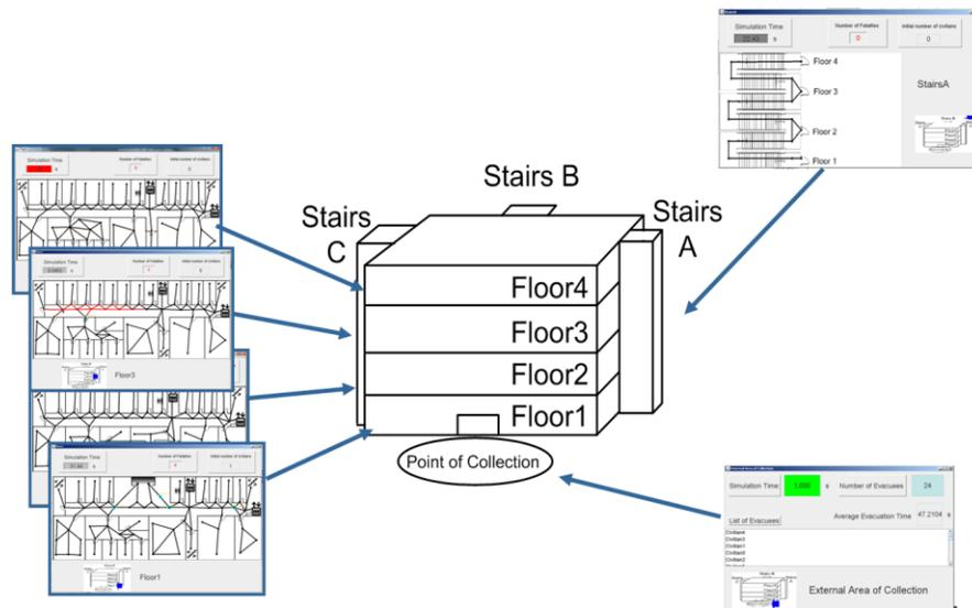
**Figure 4 Distributed Building Evacuation Simulator**
