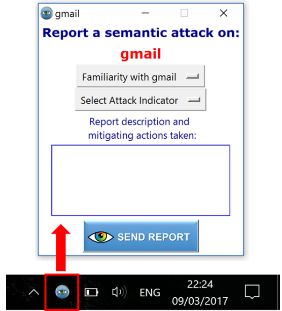
Fig. 3: The Cogni-Sense HaaS reporting app icon running in system tray. When clicked, a reporting window is opened with the detected platform and report information
