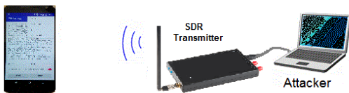
Fig. 3: Attack environment of hardware-assisted location spoofing consists of an Android phone, a laptop and a software defined radio (SDR) transmitter (HackRF)
