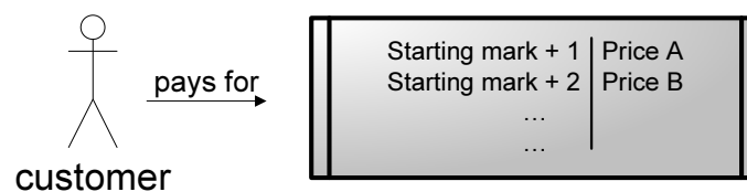
Fig. 6.4: The customer pays for an increase in the DoS mark so that his packets will have higher priority during a DoS attack (see Chapter 4 for details on the DoS mark).
